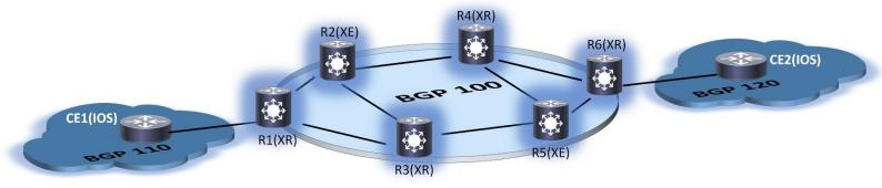
This step is to migrate to a complete segment routing topology (apart from some remaining LDP only nodes, R1, R6)
